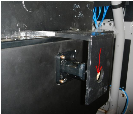
Hole in bracket where USB cable connects (left) and the two screws that attach the protective bracket (right).
