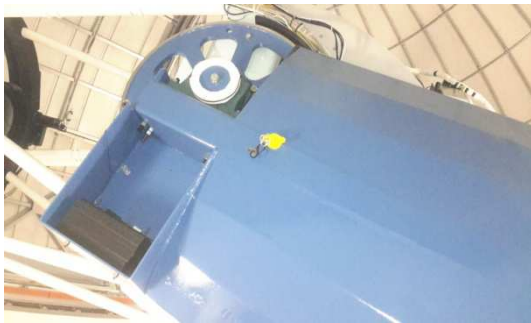
Figure 1: Safety lock pins inserted on east and west side of the fork (yellow handles)
