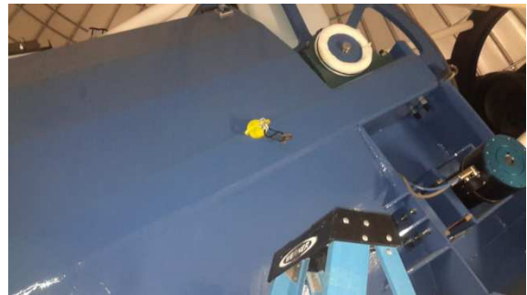
Figure 1: Safety lock pins inserted on east and west side of the fork (yellow handles)
