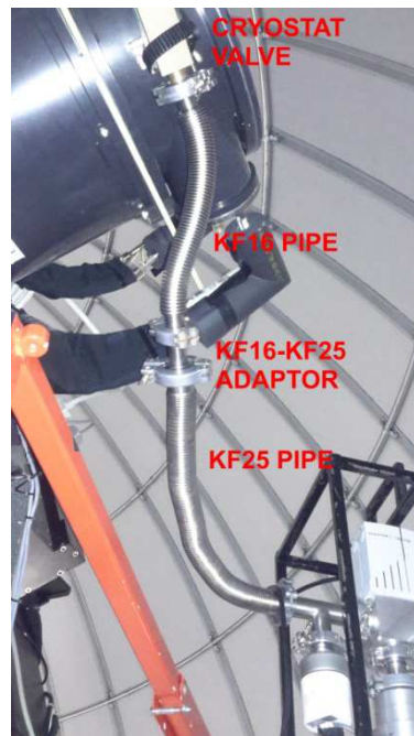
Figure 2: vacuum pump to cryostat connection fittings
