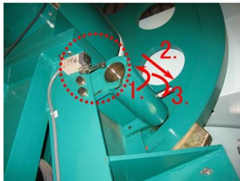
FIGURE 9: TELESCOPE SAFETY PIN ENAGAGED.
