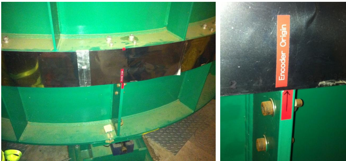
Figure 10: Encoder origin aligned
