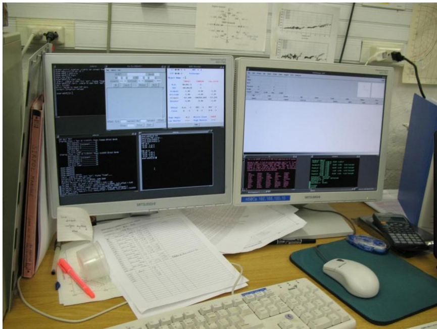
Figure 4: Sirius computer with dual-monitor display for telescope and dome operations (left screen) and detector output (right screen).
