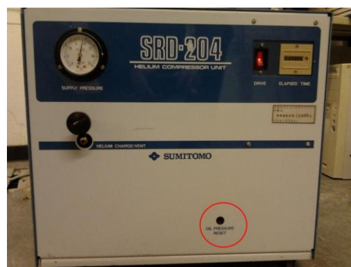
Figure 19: The Helium cooler compressor Unit
