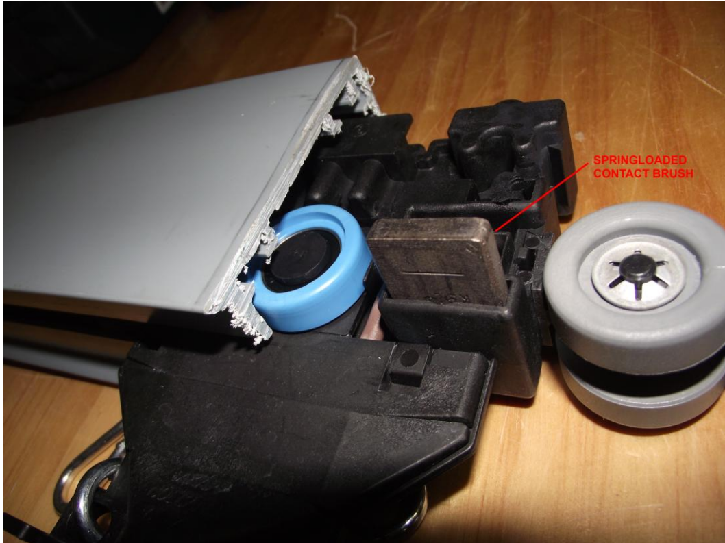
Figure 4: Dolly showing one springloaded contact.
