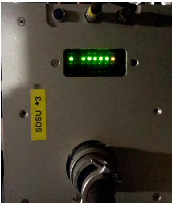
Fig. 5: SDSU Controller: LEDs all ON indicating operational mode (see note below)
