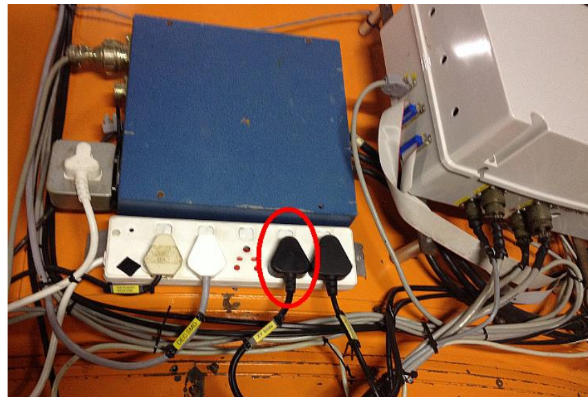
Fig. 13: Hippo XY-Slides and Instrument Selector auto-guider AUX power switch indicated
