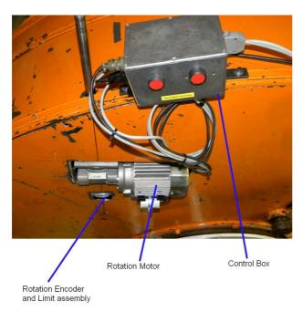
The Instrument can only be rotated from the Control box on the telescope. The instrument rotation encoder is read by the telescope control PLC and the TCS use this reading to calculate the correct auto-guider errors during guiding.
